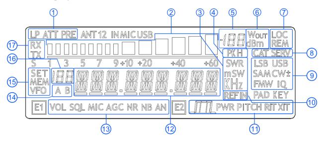
1. LP: turns on when the low pass filter is active.
