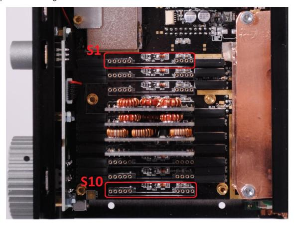
As shown in the FDM-DUOr front end block diagram below, use slots 4 to 10 for HF (under Antenna 1) and slots 1 to 3 if using Antenna 2 (no low pass filter).
